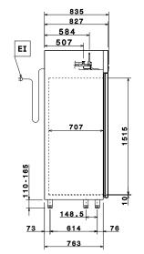
Electrical inlet (power) Refrigerant Inlet RO Refrigerant Outlet
